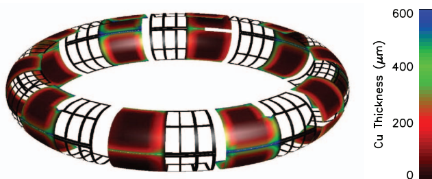
FIG. 1. The close-fitting conducting wall of the HBT-EP device. The wall is composed of 20 individual stainless steel segments, each of which is coated in copper to adjust the L/R time of the wall. Copper thicknesses shown here are based on the modeling discussed in Sec. VII.
